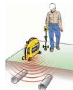
Induce a signal to locate utilities.
