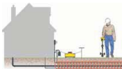
Direct connect to utility lines.
